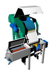
**Principle of working** The screenings fall through the feeder into the rotating screw. The screw rotation in the trough is assured by the electrical gear box. The screenings move through the screw from the feeder to the outlet from the screw. The screw conveyor can be inclined up to the angle of 30°.
