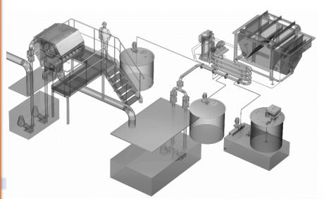
Typical technology scheme for wastewater pre-treatment - mechanical filtration by a **rotary screen** (or **drum screen**) with integrated screening press, chemical treatment by **chemical unit** dosing coagulant and flocculant, and flotation process of fine treatment by the dissolved air flotation D.A.F – **flotation unit**.
