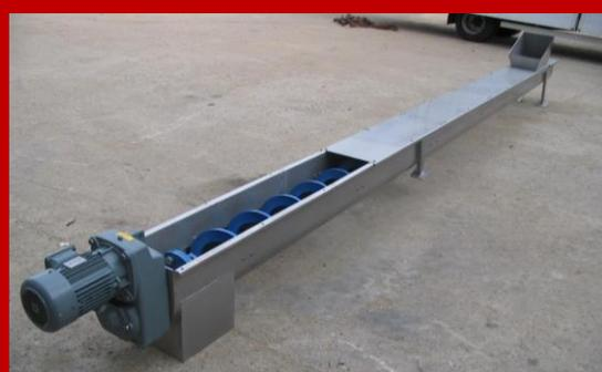
Screw presses SL are used for dewatering of the screenings from the rotary or drum screen.
